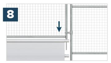
Slot the mesh fence panels into the top of the manta barriers.
