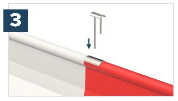
Once the barriers are in place, the connecting pin slots down through the top of the barrier to hold in place.
