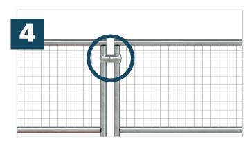
Secure the panels in place using a standard coupler.
