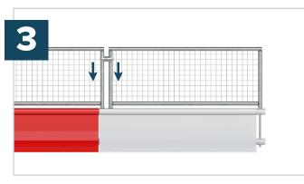
The pedestrian and vis rails/guards slot neatly into the top of the barriers and no additional pins are needed.
