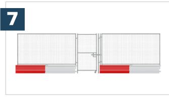
Gates can be easily added to the manta barrier system.
