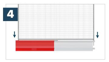
With the connecting pin in place, you can then insert the fence panel in to either end of the barriers.
